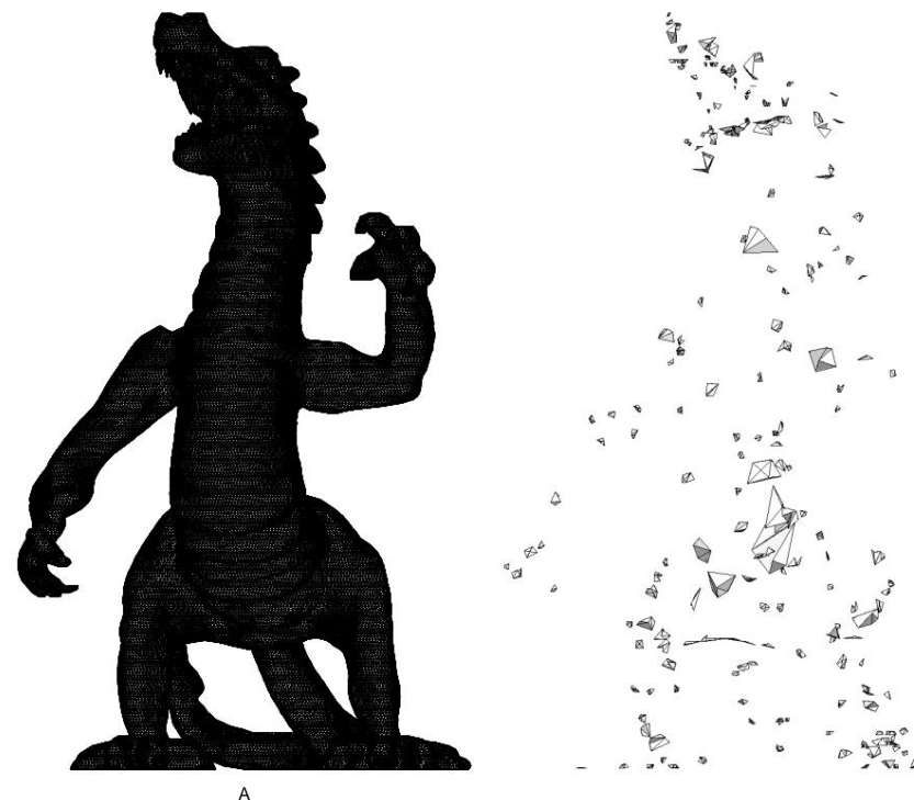
Fig. 3.20. Operation of the advanced front algorithm on the dragon model: a - initial front, b - final front
