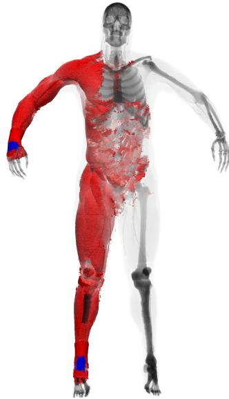
Figure 1: Sensitivity analysis of the conventional 4-electrode scheme: red zone indicate high positive sensitivity, blue zone indicate negative sensitivity. The skeletal bones are added to the image to improve perception.
