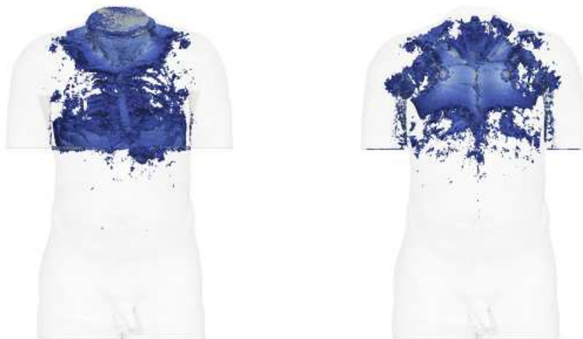
Figure 7. Areas of high sensitivity providing 70% of the whole sensitivities. Measurement frequency 50 kHz.
