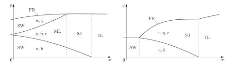
Water waves: mixing layer, near-surface turbulent layer, turbulent bore. Gas dynamics: pseudo-shocks.
